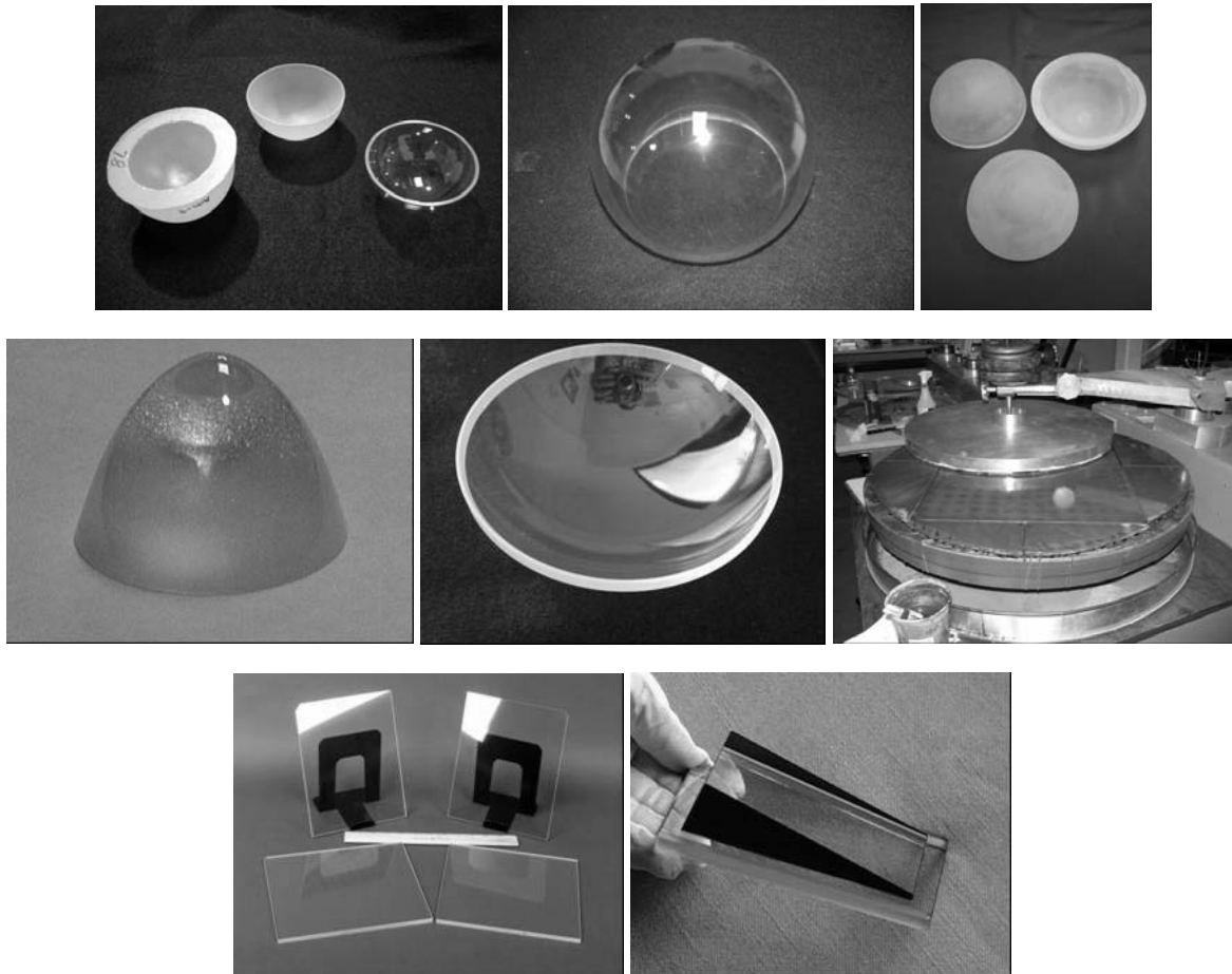
Figure 4. Examples of ALON optical components produced by Surmet.
