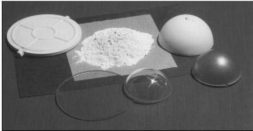
Figure 1. Prototype ALON missile launch tube windows and domes, at various steps of manufacture. Powder → Injection molded components → Heat treated components → Finished window and dome
