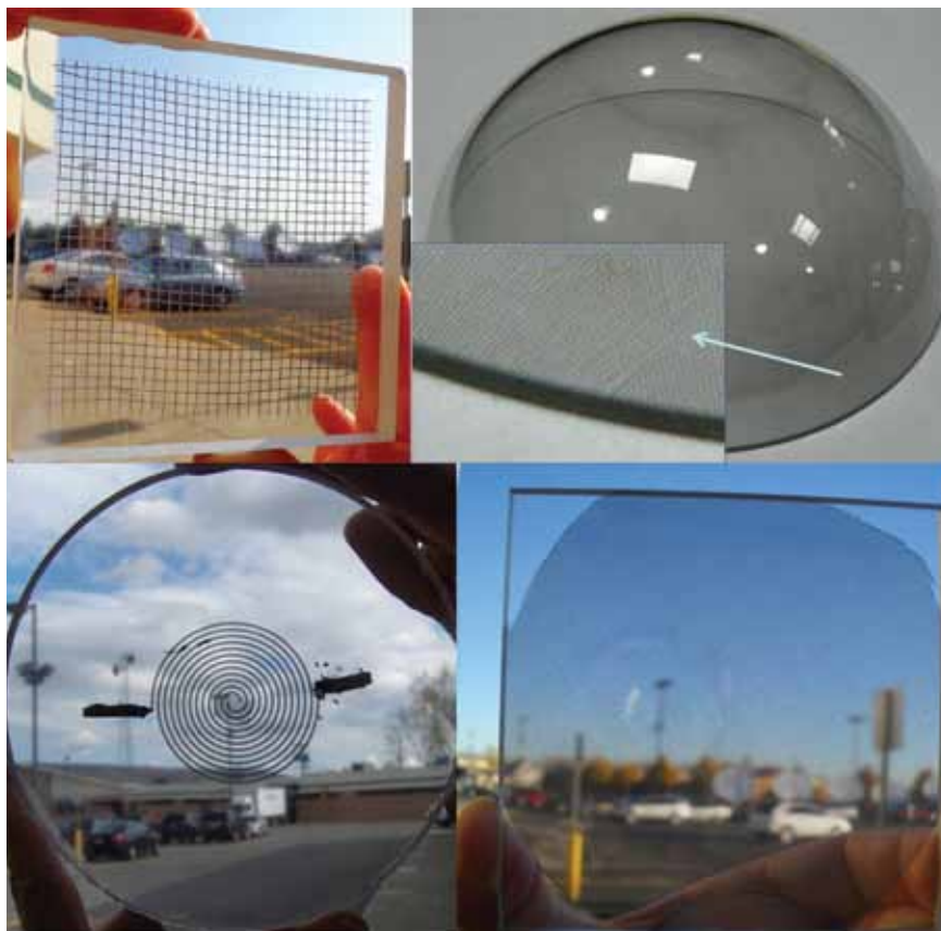
Figure 4. Examples of ALON components with embedded internal architectures.
