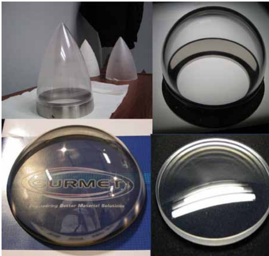
Figure 3. Examples of ALON and spinel components with complex geometries.
